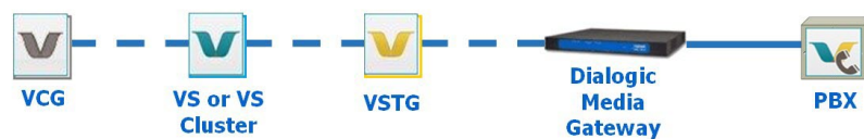
Figure 2: VSTG connecting to PBX through Dialogic Media Gateway
