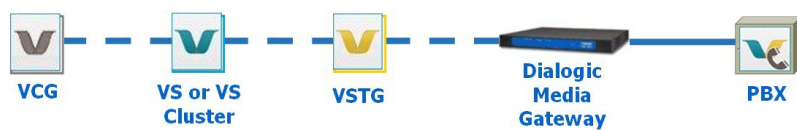
Figure 2: VSTG connecting to PBX through Dialogic Media Gateway
