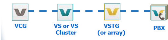
Figure 15: Vocera software installed on separate computers
