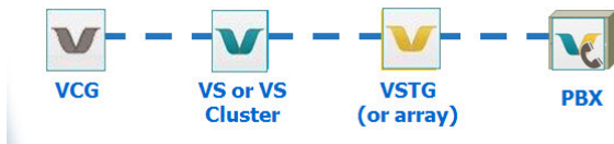
Figure 3: Vocera software installed on separate computers
