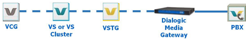
Figure 8: VSTG connecting to PBX through Dialogic Media Gateway
