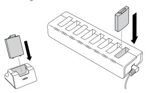
If battery capacity exceeds 80%, the blue indicator light will turn off after a second. The green indicator light on the front of the charger will begin to blink when the battery is positioned correctly, and it will continue to blink while the battery is charging. When the indicator glows steadily, the battery is fully charged. Charging normally takes only a few hours.
