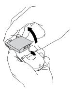
2. Insert the battery into the charger, and press down on the battery until you see the blue indicator light turn on.
