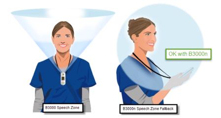
It is still recommended to wear the B3000n badge in a position that directionally uses the array of microphones. But the automatic Speech Zone Fallback mechanism alleviates some of the difficulties with voice recognition when the B3000n is orientated incorrectly.
