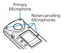
The noise cancellation features of the B3000 badge have been designed to provide a significant improvement in speech recognition accuracy in environments with background noise.
