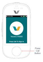
A small haptic feedback vibration is felt when the button triggers. The **Call** button must be operated with bare fingers, light gloves, and through thin clothing. The button will not trigger if you are using thick gloves or thick clothing.
