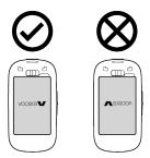
Do not insert the battery backwards and upside down as shown in the image below:
