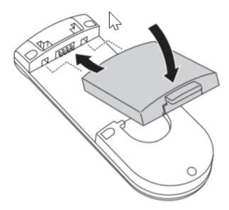
4. Slide the pegs at the top of the battery into the two holes in the Badge's battery compartment and press down gently to seat the battery in the Badge.
