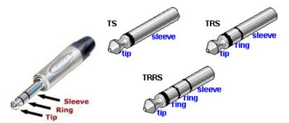
Typically the TRS connecter is mated to a headset which contains a speaker and microphone. If the headset is a monaural headset (one ear piece), the TRS connector is used. If the headset is a binaural or stereo headset, a TRRS connecter is used which contains one extra Ring for the second earpiece.
