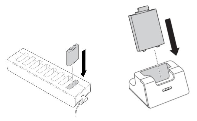
3. When the green light stops blinking and is steady, the battery is fully charged. Remove it from the charger.
