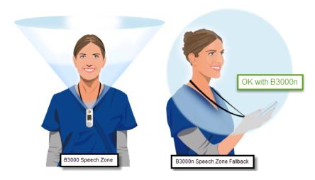
It is still recommended to wear the B3000n badge in a position that directionally uses the array of microphones. But the automatic Speech Zone Fallback mechanism alleviates some of the difficulties with voice recognition when the B3000n is orientated incorrectly.
