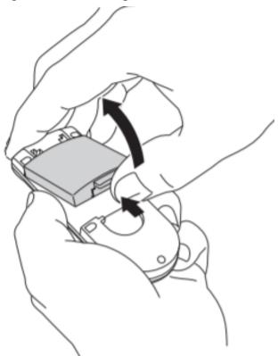
2. Insert the battery into the charger, label facing back, and press down on the battery until you see the blue light turn on. After a second, the green light will begin to blink. **Note**: If the blue light remains on and is steady, the battery is beyond its useful life. If so, replace it.
