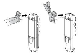
You also can connect the lanyard or clip to the badge before installing the battery.
